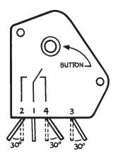
Some refrigerators such as GE do not incorporate connectors for a defrost timer hook-up. Each terminal is connected using a seperate wire. In this case, very carefully bend terminals 2, 4, 3 as illustrated. Use needle-nose plier to hold the terminal while bending it with another plier.
